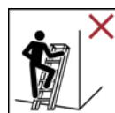
Standing ladders shall not be used as a leaning ladder unless it is designed to do so.
