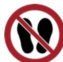
The part of the ladder with this sign is not allowed to stand on.
