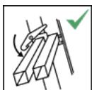
Locking devices shall be checked and be fully secured before use if not operated automatically.
