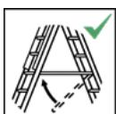
Use the ladder with restraint devices engaged only.
