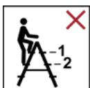
Do not stand on the top two steps/rungs of a standing ladder without a platform and a hand/knee rail.
